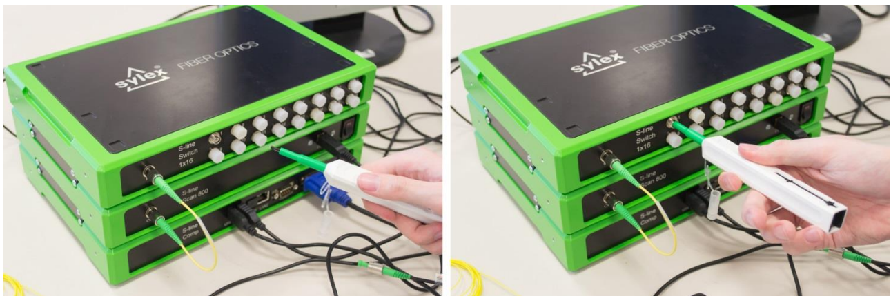
Figure 1: Cleaning the connector inside the adapter
