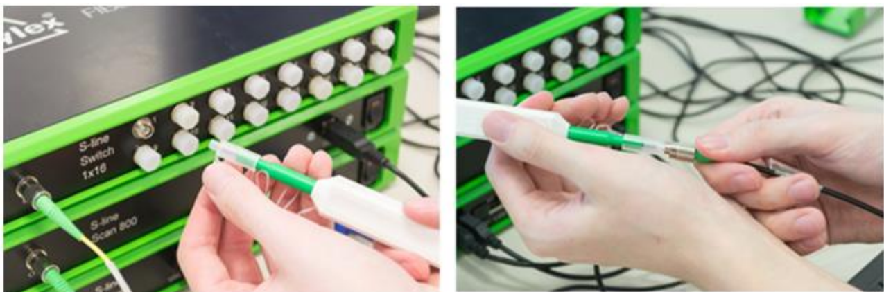
Figure 2: Cleaning the free end connector
